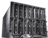
Dell PowerEdge M1000e Chassis M620 Blade Server
